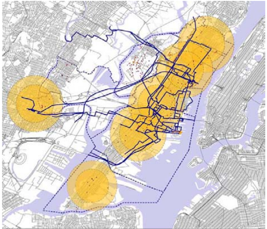
Overlapping broadband infrastructure in Hudson County - includes fiber network, DSL service areas and cell towers
